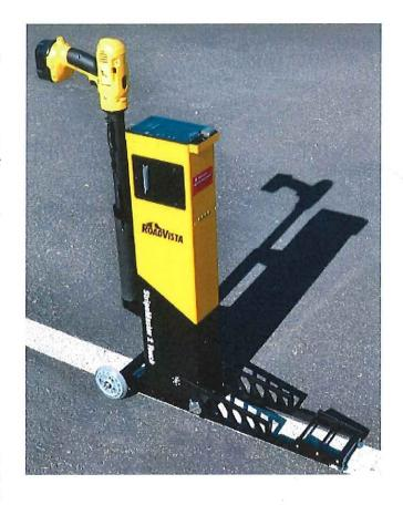
Measurements can be made in 0.2 seconds and the instrument is ready for the next measurement in less than 2 seconds. This means the user spends less time on the road, which increases worker safety. The SM2-Touch can measure profiled markings up to 0.59 inches (15 mm) in height.
