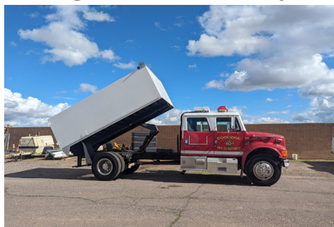
Newly converted 5-yard dump truck, image courtesy of City of Coolidge Public Works
